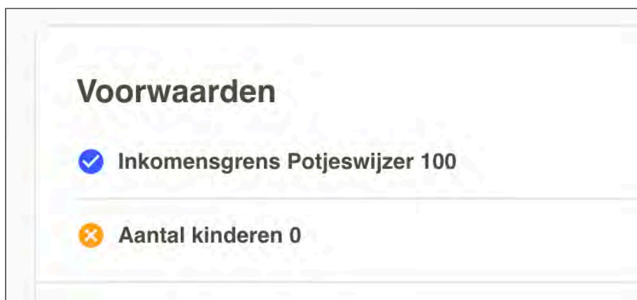
Figuur 4: the orange icon has low contrast and the images have no alternative text
